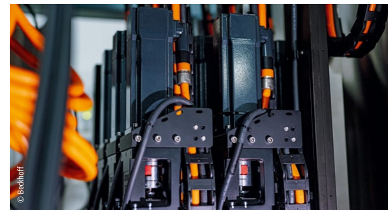
Beckhoff AM8100 servomotors with ball screw actuators to raise and lower the PECM tooling with maximum precision.
