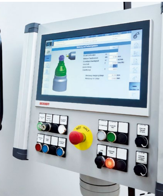
The tools and jobs are selected via a CP2916 multi-touch Control Panel, which is connected to the CX5140 Embedded PC in the control cabinet.
