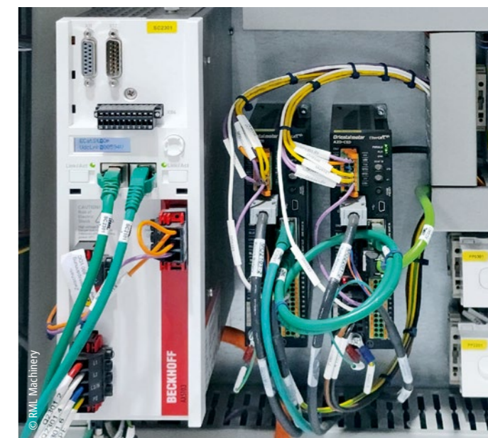
An AX5103 servo drive with AX5805 TwinSAFE option card provides precise and reliable movements.
