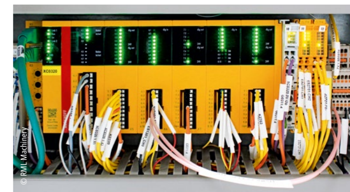
The EK1960 TwinSAFE Compact Controller ensures functional safety.
