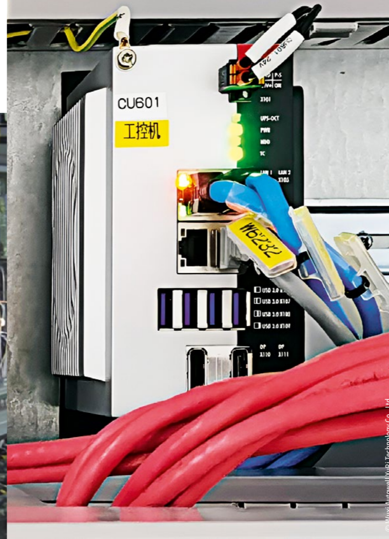
The open and flexible ultra-compact C6030 Industrial PC controls a great variety of third-party devices acting as slaves in the EtherCAT automation network.
