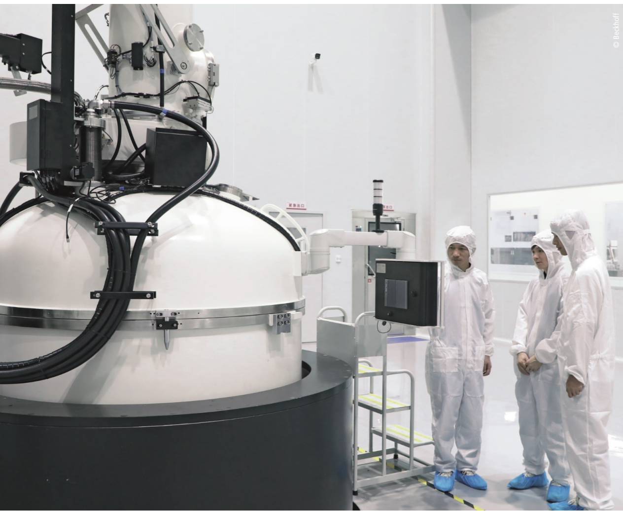
Prerequisite for growing high-quality monocrystalline semiconductors is continuous furnace operation in intervals of several days through to two weeks.
