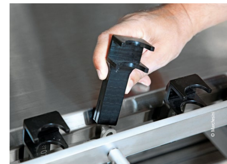
During a product change, the plug-in bottle holder design enables the carriers for the XTS movers to be adjusted just as quickly as the pre-configured motion profiles are called up via the HMI.
