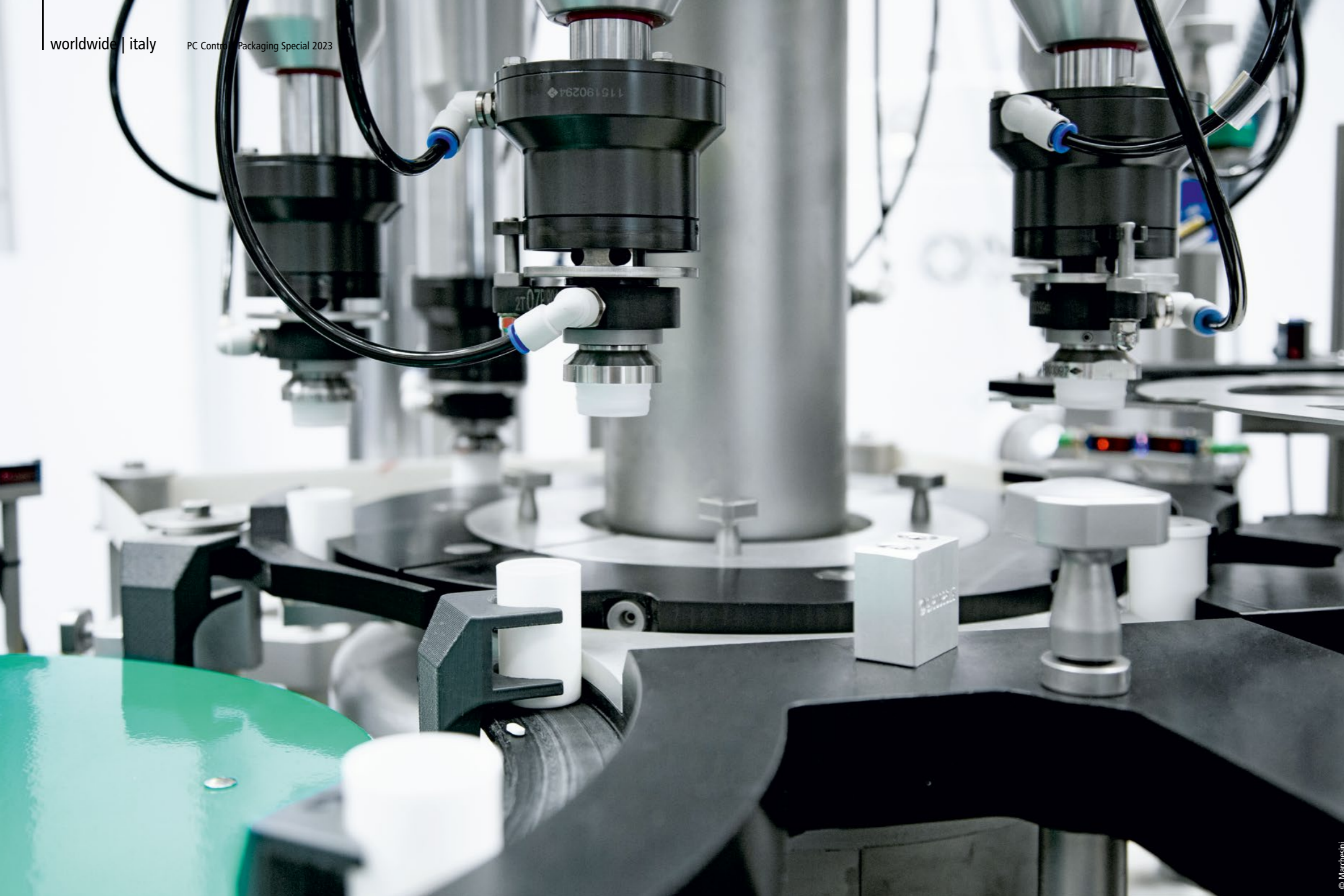
With their interchangeable bottle holders, the individual XTS movers can synchronize accurately with the capping unit turret.
