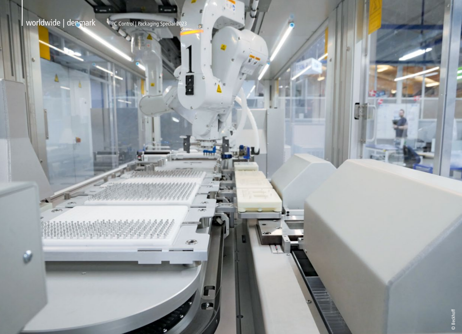
Product insertion into a blister transported by a XTS mover
