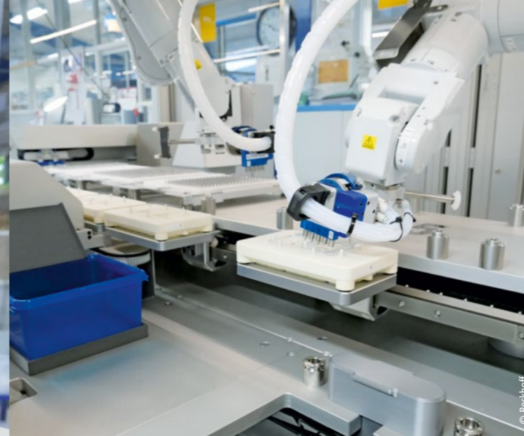
Product insertion into a blister transported by a XTS mover
