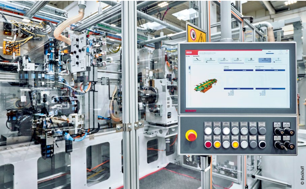
The CP3918 multi-touch Control Panel, together with a specific push-button extension and the convenient user interface created with TwinCAT HMI, enables optimum use of all machine functionalities.
