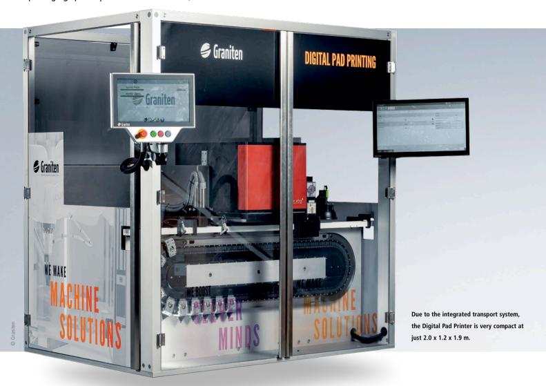
The eXtended Transport System at the core of a digital pad printing machine for the pharma industry
