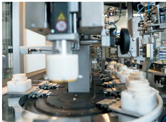
The compact machine for closing cosmetics containers is based on XTS technology.
