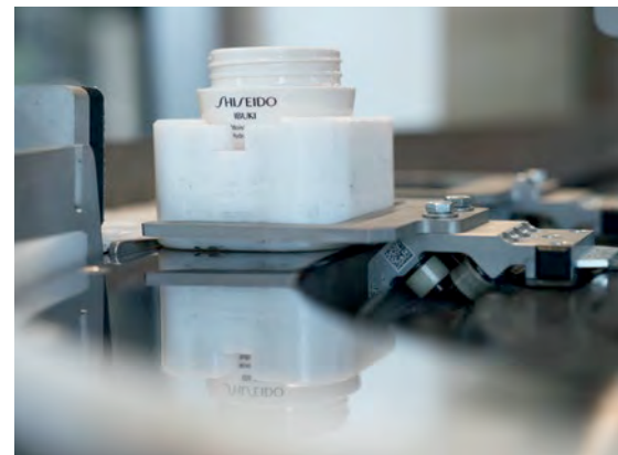
The individually and precisely controlled product transport with XTS makes sure that the high-quality Shiseido cosmetics containers are handled without any damages.
